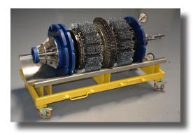
Optionally, the MFL tools can be equipped with tri-axial sensors for even better detection and sizing. Tools of other sizes and higher performance specification are available upon request.
